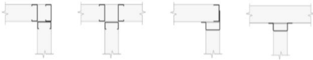
Fig. 3.5 Corners and junctions showing examples of stud positions and fixings
